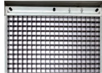
Flowing vertical ice making Evaporation temperature: -18^{\circ}\text{C} Ice center temperature: -13^{\circ}\text{C}
